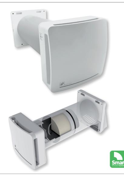
Decentralized ventilation unit, with heat recovery, for single rooms in domestic or commercial applications. Elegant design that allows its adaptation to any environment. Brushless motor with low comsumption electronic control. Ventilation system through an reversing motor and a heat exchanger with a performance up to 93%. Designed for a continuous operation, the unit adjusts the airflow proportionally to the humidity level (model RD), ensuring excellent indoor air quality.
