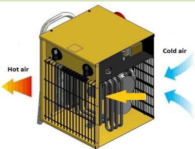
The device works on the principle offorced convection . The air flow is forced fan. Cold air is drawn in the back of the unit. Further washes flowing from the heater receives heat. The heated air is expelled in front of the heater. The device has a thermostat for the regulation temperatures 5-35  $^{\circ}$ C. The unit area equipped with thermal protection is acting automatically. The unit features: ventilation, heating with half the power, heating at full power. Device has cooling thermostat.
